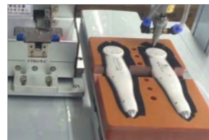
Small appliance lock screw
